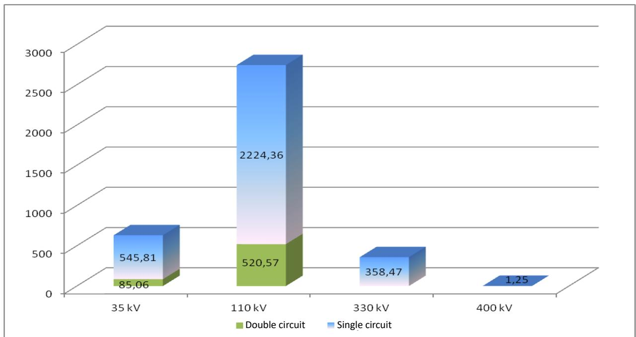
**Figure 2.11** The rate of OHLs with concrete pylons
