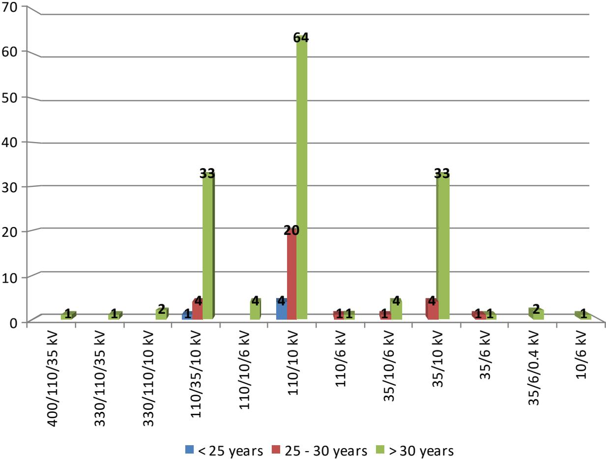
**Figure 2.3** The operation period of TSO’s electrical substations
