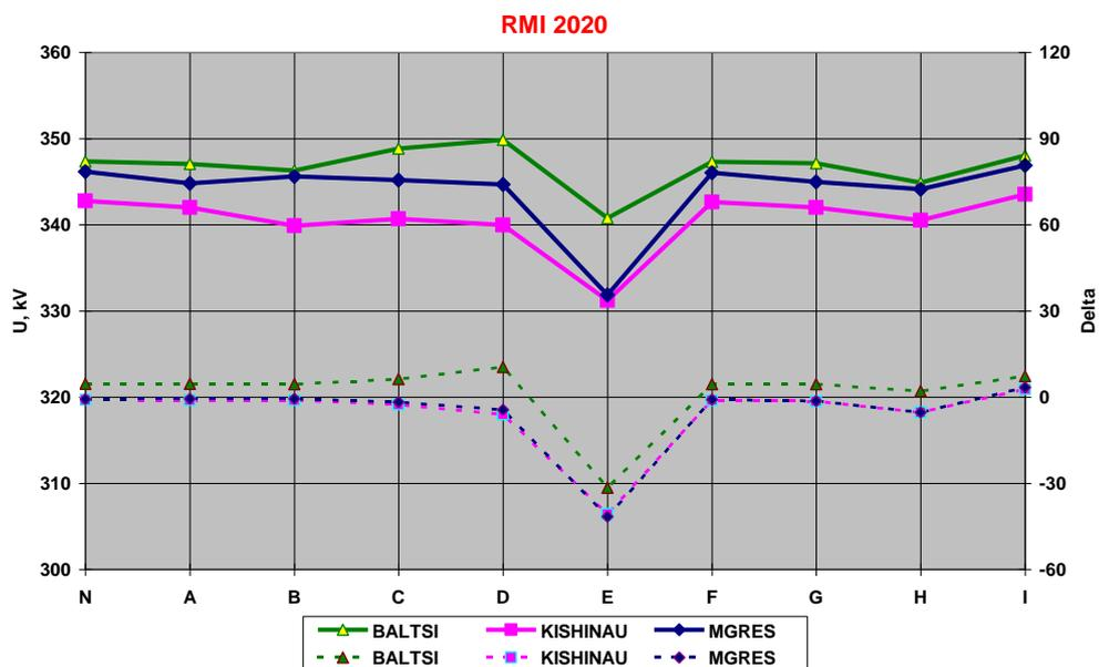
Figure 4.2 Voltages and angles in transmission grid nodes, with N-1 elements in operation, for calculation model for year 2020
