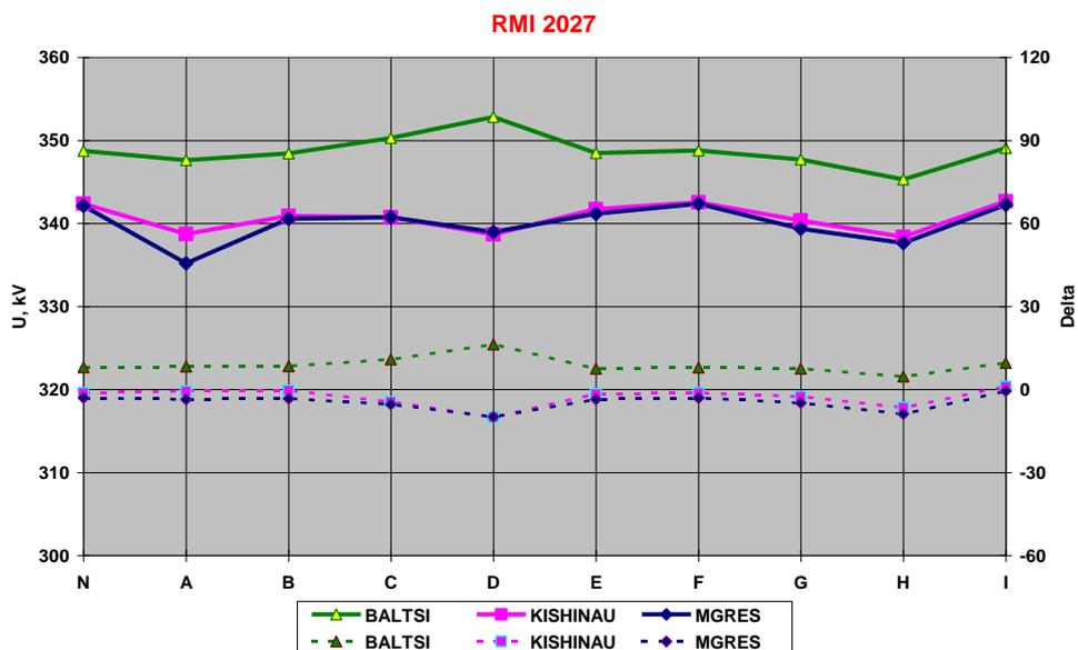
**Figure 4.4** Voltages and angles in transmission grid nodes, with N-1 elements in operation, for calculation model for year 2027
