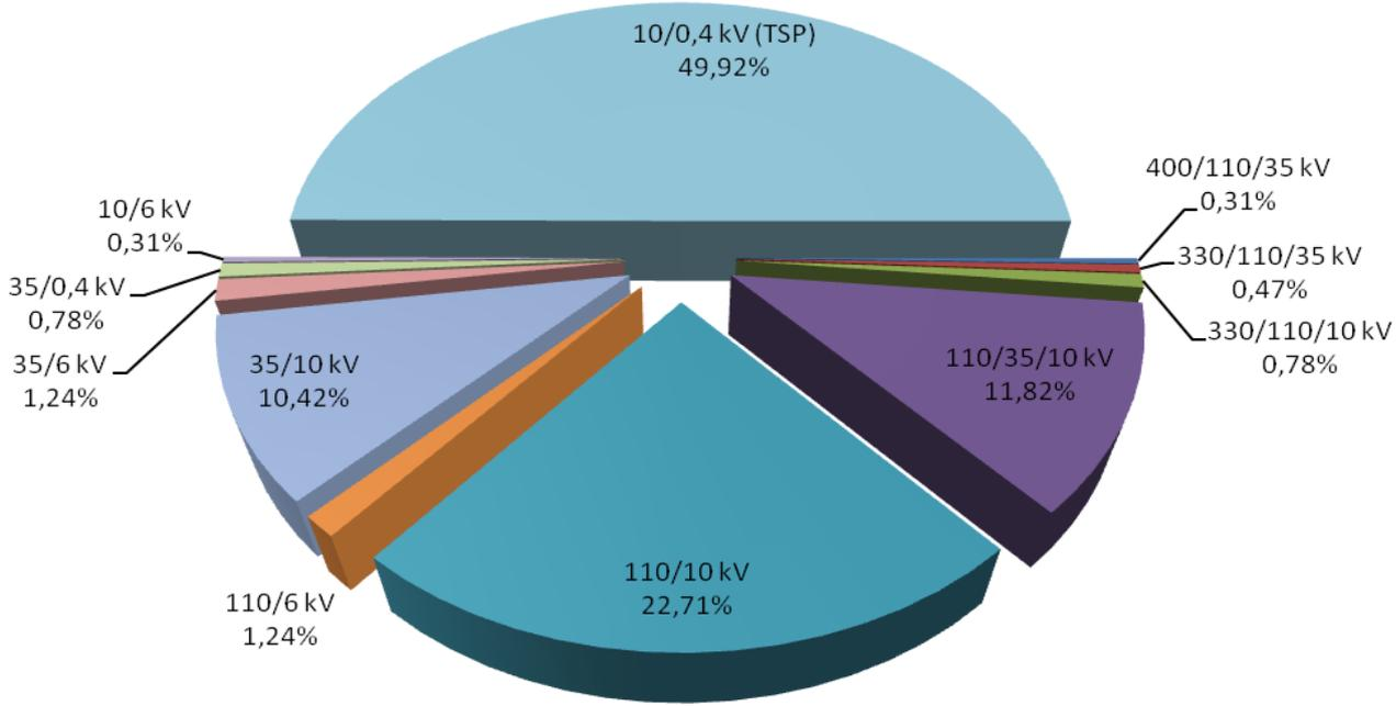
**Figure 2.5** The rate of the power transformers from TSO's electrical substations
