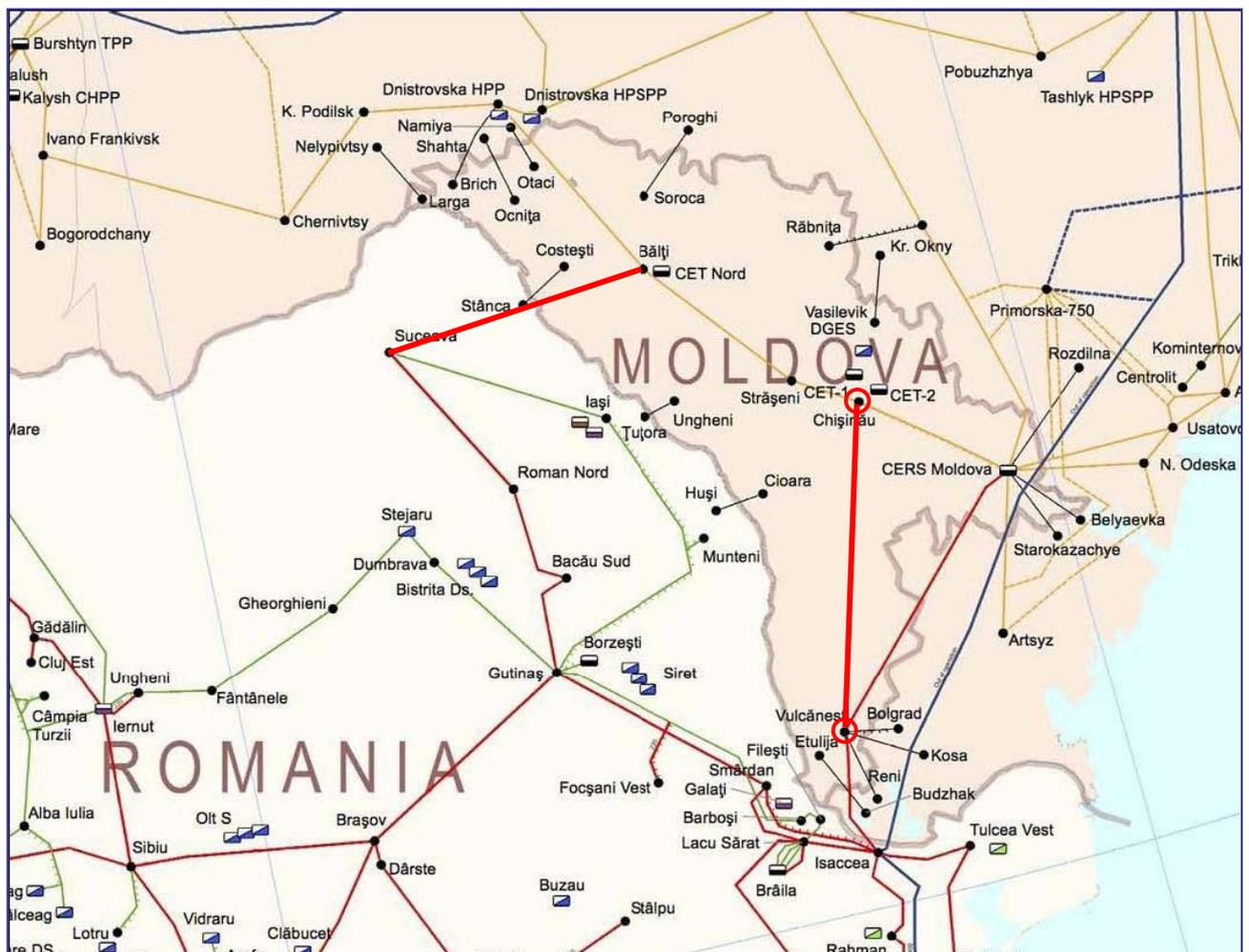
**Figure 3.3** Scenarios regarding construction of interconnection lines
