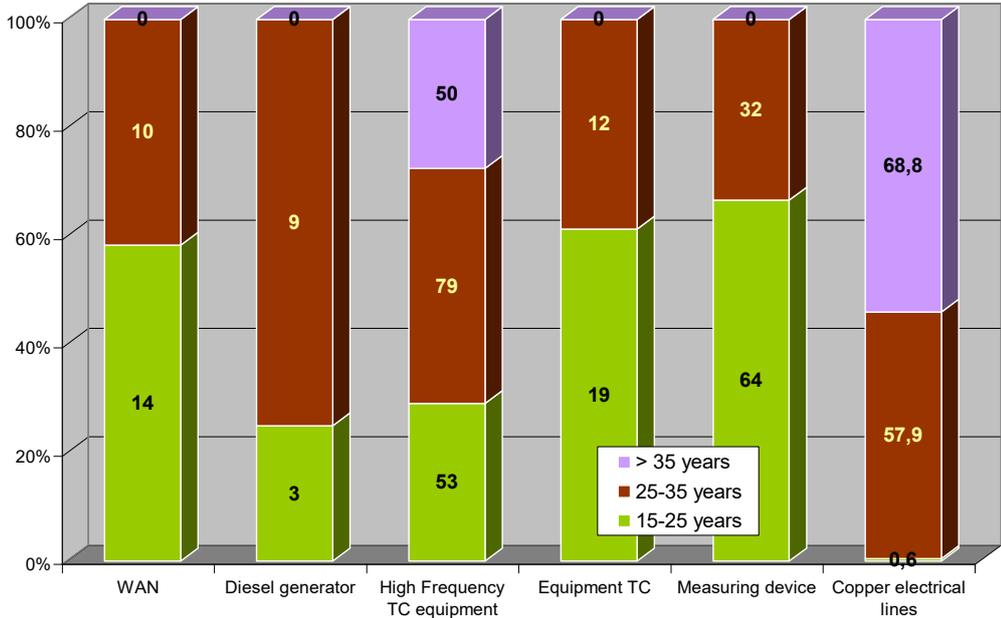
**Figure 2.16** The information about telecontrol equipment of TSO’s electric transmission network
