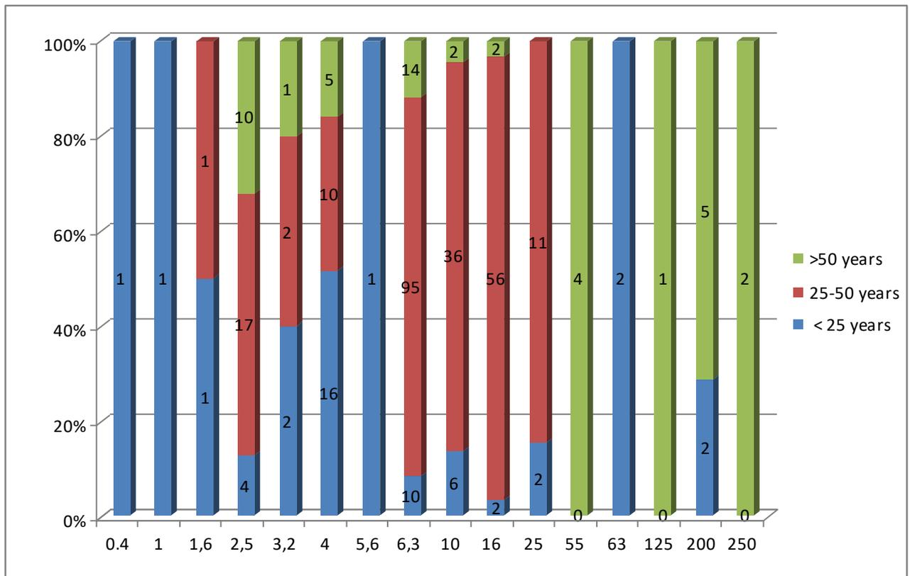
**Figure 2.4** Operating period of TSO's power transformers.
