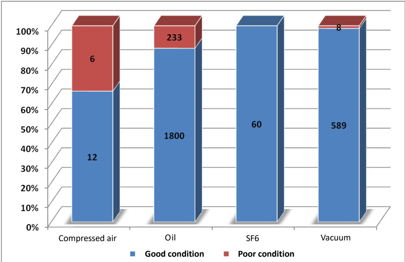
**Figure 2.6** TSO's circuit breakers technical state
