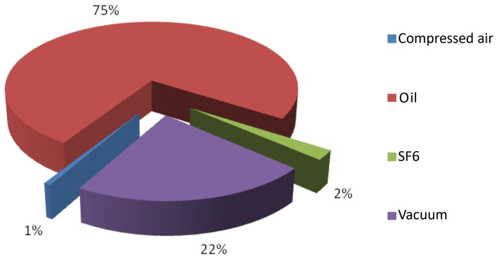
Figure 2.7 The rate of the 10-400 kV TSO's circuit breakers
